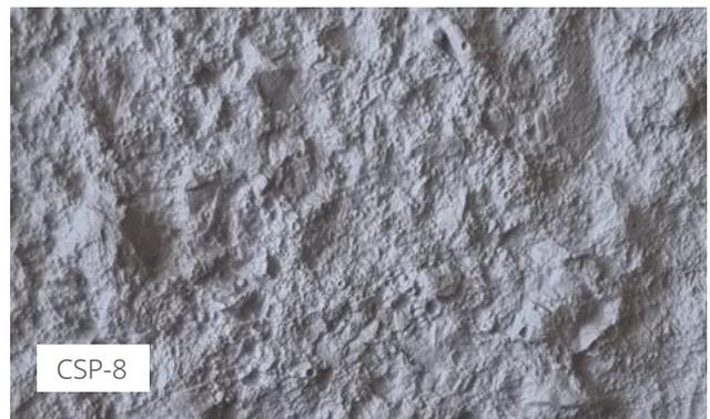
Suitable surface preparation methods are grinding, high-pressure water blasting (at least 350 bar) and sandblasting/shotblasting.
