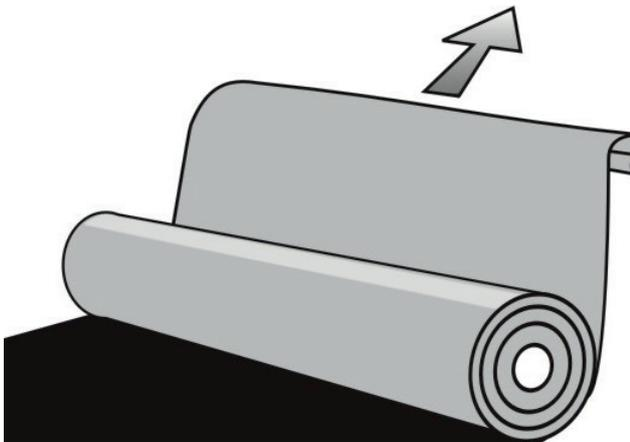
Continue to pull off the backing paper evenly when progressing to bond the KÖSTER KSK Membrane to the substrate without folds and without enclosures of air.
