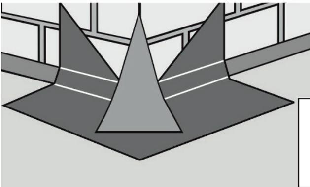
Then bond a triangular shaped piece of membrane onto the corner with the tip pointing upwards.
