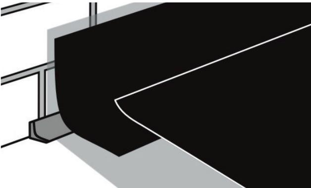
Apply the KÖSTER KSK Membrane onto the floor, overlapping onto the previously installed strip of membrane.
