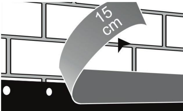
Seal the upper edge including the nails with KÖSTER Butyl Fix-Tape Fleece. The tape can be plastered over.
