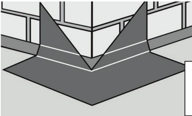
Outside corner: First bond a diagonally cut piece of membrane to the substrate in the corner.
