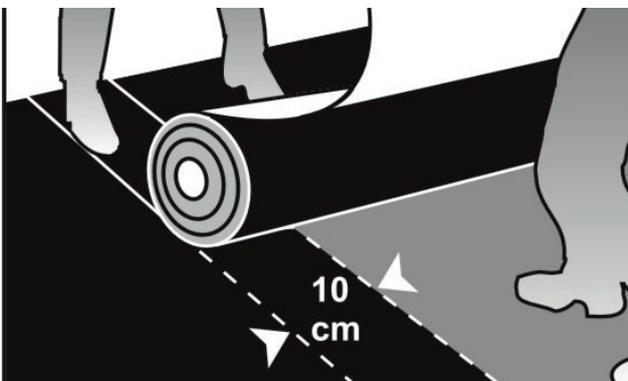
When applying the membrane overlap individual sheets by at least 10 cm.
