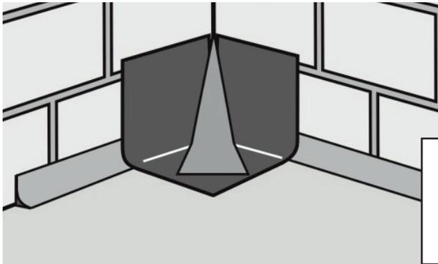
Then bond a triangular shaped piece of membrane onto the corner with the tip pointing upward.
