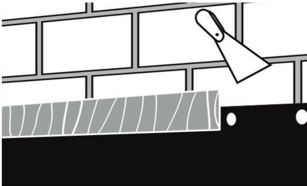
After fastening, the upper seam must be secured against leaking from behind. To do this, the area should be filled with KÖSTER KBE Liquid Film.
