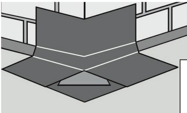
Finally apply a piece of membrane cut on the side as shown.
