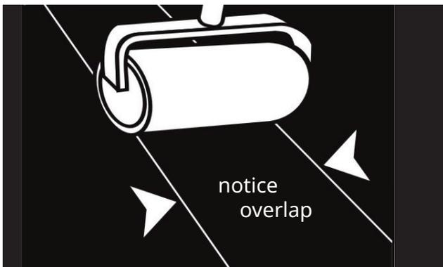
Sheets of membrane are placed so that the edges on longitudinal and transverse seams overlap by approx. 8 cm and at connections 10 cm. Use a roller to firmly press the membranes onto the substrate. On overlapping areas, take special care to ensure that the membranes have been pressed together well. When used for sealing in and under walls, the overlap must be at least 20 cm. The waterproofing according to DIN 18 534 is carried out in one layer up to water exposure class W2-I.
