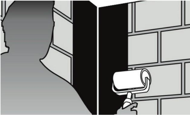
On inside corners, apply a piece of membrane at least 30 cm wide into the corner area.
