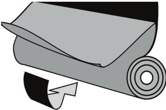
Pull the backing paper through underneath the roll and bond the exposed adhesive side of the membrane to the substrate.
