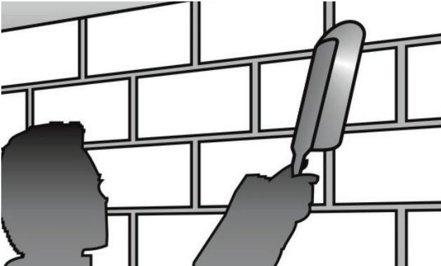
Remove loose particles. The substrate must be clean, sound and solid, free of oil and grease and other substances that may inhibit adhesion.
