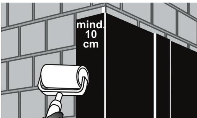
Apply the membrane on corners to the substrate on both sides of the corner by at least 10 cm.
