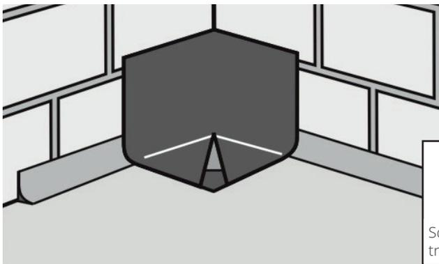
Finally, apply a piece of membrane with the triangular shaped cut out as shown.
