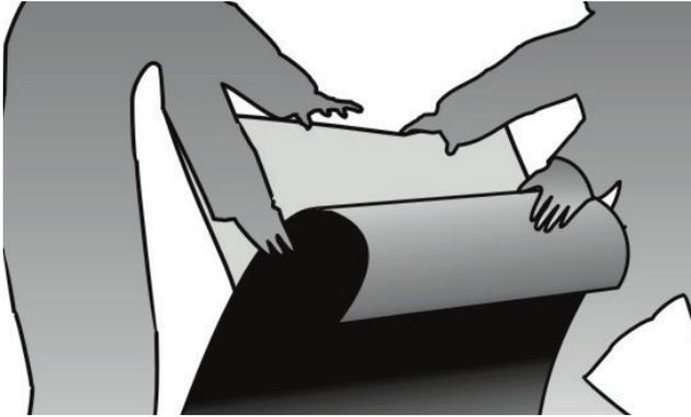
Pull the backing paper off on a length of 20 cm.
