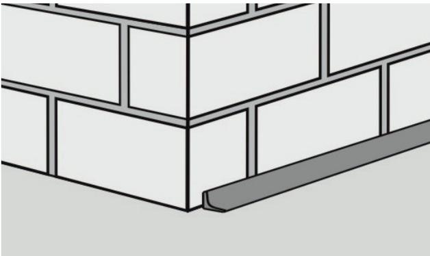
Round out edges. Install fillets in the wall / floor junction using KÖSTER WP Mortar. Close voids and holes using KÖSTER WP Mortar.
