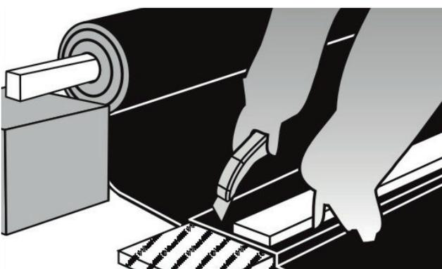
Cut the KÖSTER KSK Membrane using a sharp knife. Cut on top of a wooden board and use a straight edge as cutting support. Wet the blade repeatedly to avoid soiling the blade with bitumen.
