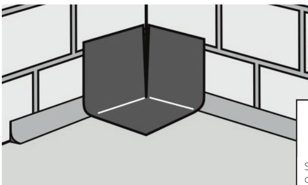
First, bond a piece of membrane with the square shaped cut out to the substrate in the corner.
