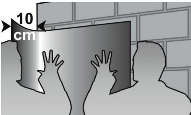
Remove the backing paper on a length of approx. 20 cm, align the KÖSTER KSK Membrane and apply it to the substrate.
