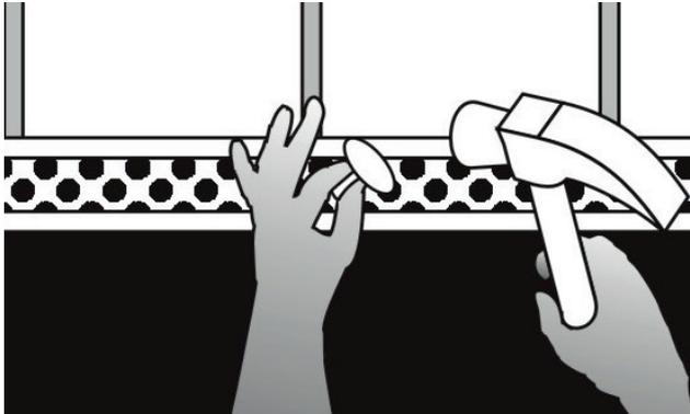
Alternatively, it is possible to use pre-perforated metal profiles for fixing the upper edge of the KÖSTER KSK Membranes in position. Also in this case, KÖSTER KBE Liquid Film is used to protect against leaking from behind.
