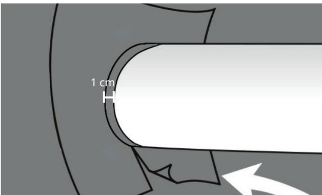
Cut a hole with the diameter 2 cm smaller than the pipe into a piece of the KÖSTER KSK Membrane and bond it to the substrate, ensuring that no air is enclosed under the membrane. If the pipe penetrations are already connected, cut the blank on the side and pull it around the penetration. Always glue the edge of the cut to the opening by at least 1 cm.
