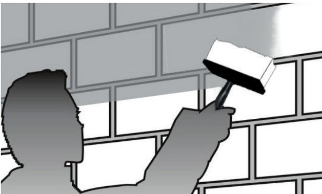
The surfaces have to be coated with KÖSTER KBE Liquid Film, diluted 1:1 with water using the KÖSTER Brush for Liquids. Mixture: 200 g/m<sup>2</sup> KÖSTER KBE Liquid Film plus water. Alternatively, the KÖSTER Primer BL with 150 g/m<sup>2</sup> can be used undiluted. In case of absorbent substrates the consumption can be higher.
