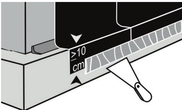
Seal the lower edge with KÖSTER KBE Liquid Film.
